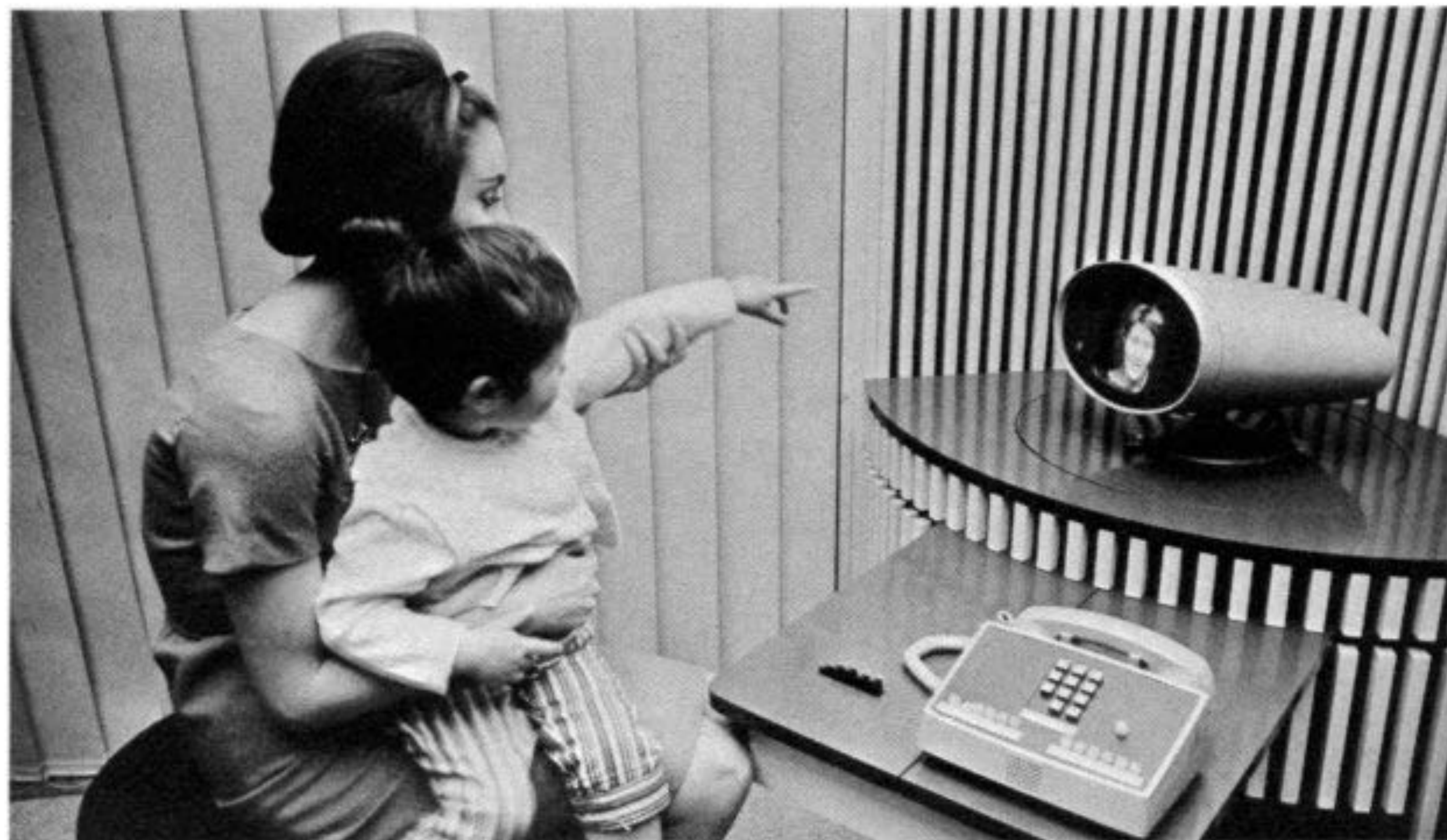
Picturephone® installation showing Touch-Tone® control console.
